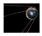
Union. The Russian word "Sputnik" means "companion". The Sputnik 1 satellite was a 58 cm-diameter aluminium sphere that carried four whip-like antennas that were 2.4-2.9 m long. The antennas looked like long "whiskers" pointing to one side. The spacecraft found out information about the density of the upper layers of the atmosphere.
